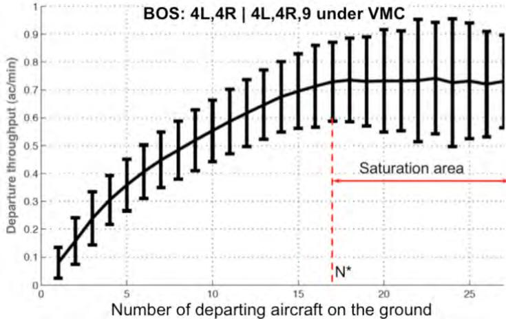
Boston Logan Airport departure throughput as a function of the number of departures post-pushback. We note how the departure throughput initially increases, but saturates once the number of departures on the ground exceeds 17 aircraft. The vertical bars denote one standard deviation.
